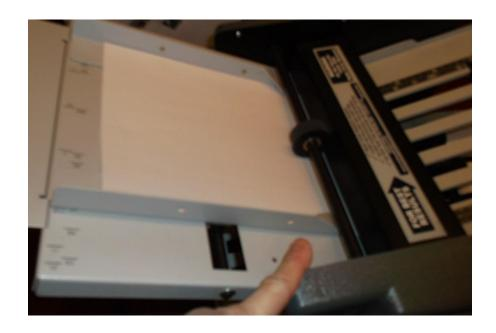
While holding the bypass lever insert the set of documents.
